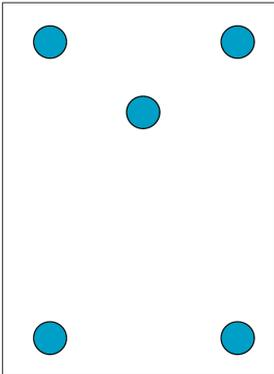
2. Now use the 5mm drill bit to make a hole 55mm deep in each of the marked fixing holes
