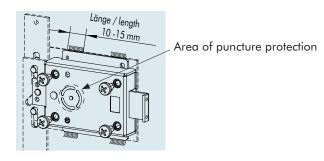
• The puncture protection should not be obstructed by other components.
