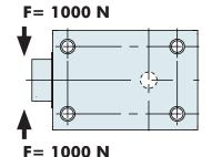
• The load on the bolt must not exceed 1000 N.
