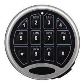
The lock when first used will be set to its default code 1-2-3-4-5-6. Enter the 6 digit code, each entry will be accompanied with a beep and a final single beep when the correct code is used. Multiple (3) beeps at the end of the code indicates incorrect code. Once the correct code has been entered move the handle from a horizontal to downward vertical position and gently pull to gain access.
