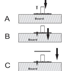
Step 3. Place the safe down over top of the anchor and fasten with the Allen bolt.
