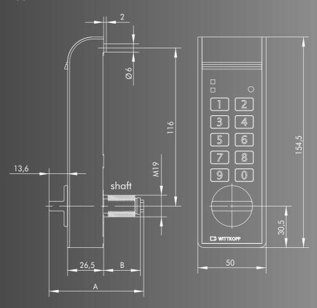
A (mm) B (mm) Suitable for door thickness
